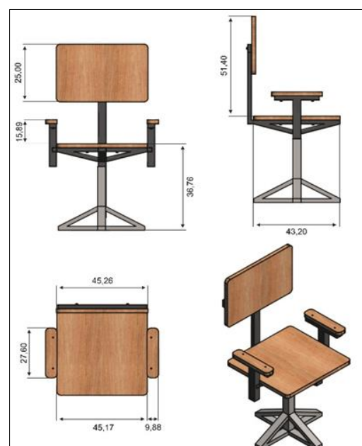
Fig 3: Chair design for a sewing business based on worker anthropometric data
