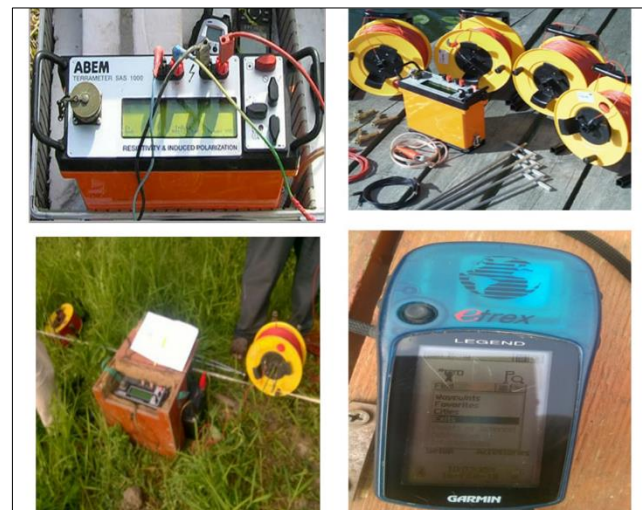
Fig 5: Abem Terrameter and accessories (a. typical Abem Terrameter b. Typical accessories c. Abem Terrameter (SAS 1000) used in this study, d. Garmin etrex GPS used in the study).
