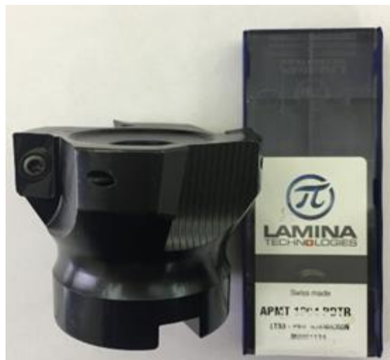
Fig 2: Milling head and carbide inserts used in the hard milling experiment
