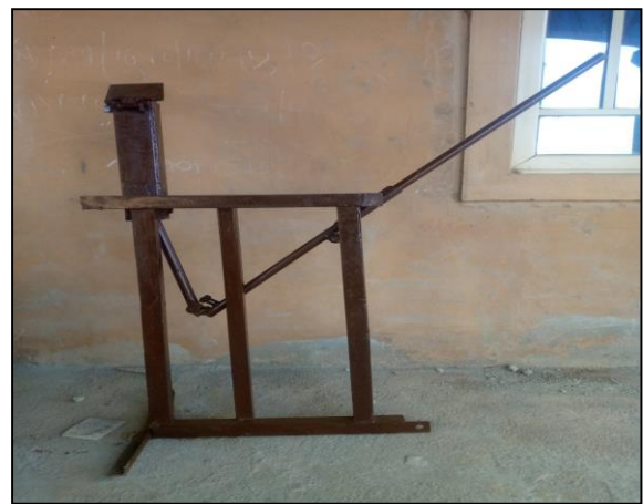
Fig 1: Locally Fabricated Hydraulic Press Briquette Moulder
