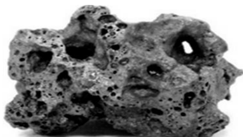
Fig 3: Macro-view of an iron ore sinter (Nicol et al. , 2019) [23]
