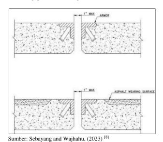
Fig 1: Butt Joint
