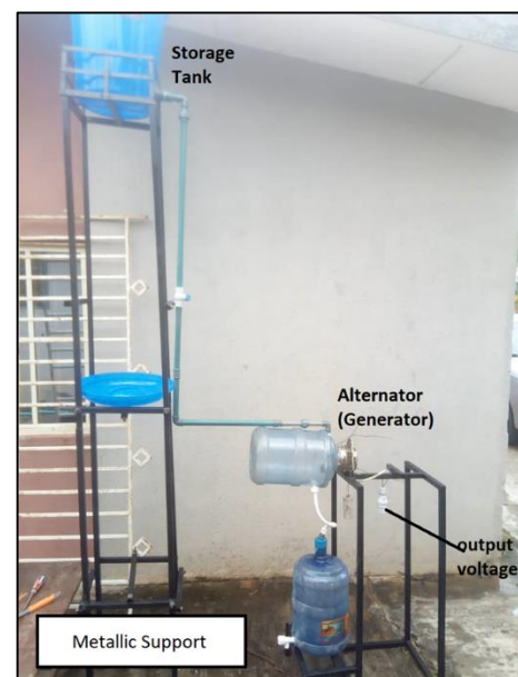
Fig 2: Complete arrangement of the mini hydroelectric power plant
