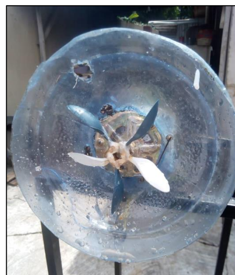
Fig 3: Designed blade for the mini Hydro-Electric power plant
