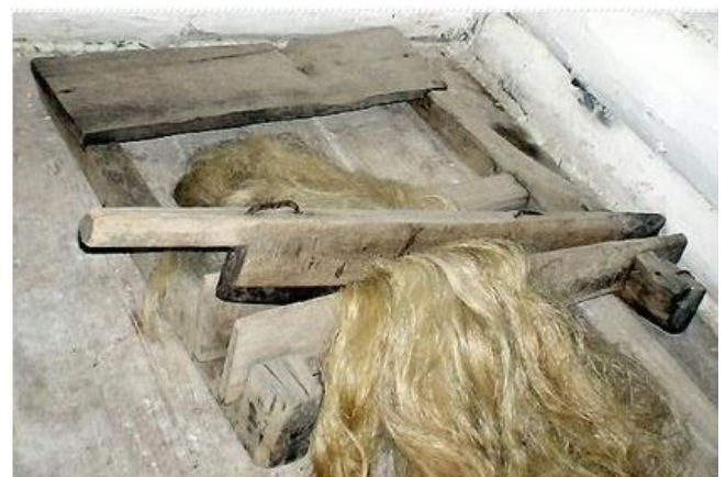
Fig 27: Traditional processing of flax ('trlica'), Godjenje village in Bosnia and Herzegovina (Geographic coordinates: 43°59'47.12"N, 19°05'47.86"E, Elevation 880 m)
