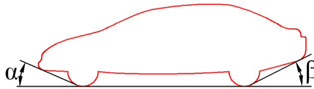
Fig 3: Car shape with front and rear maneuverability angles
