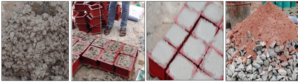
Plate 3.4: Showcasing the mixture of laterite concrete cubes specimen
