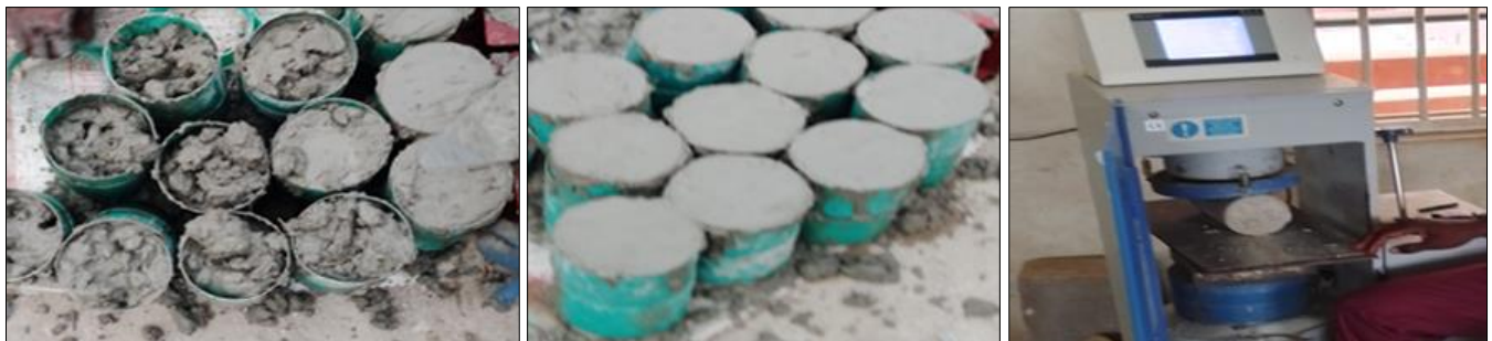
Plate 3.5: Splitting tensile strength concreting process
