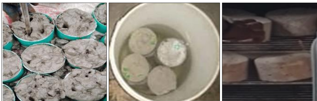
Plate 3.5: Various sections of sorptivity and water absorption laboratory test.
