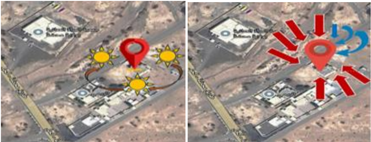
Fig 1: Sun and Wind Orientation Analysis highlighting natural ventilation opportunities.
