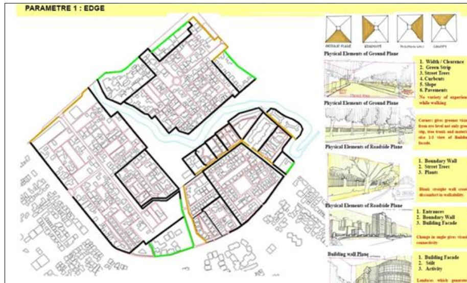
Fig 9: The edges of the periphery of gated developments are into 3 categories. The categorization of edges are done with respect to physical elements in 4 planes.
