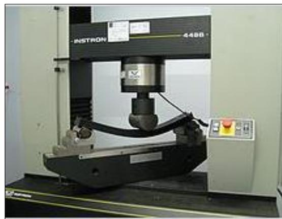
Fig 6: Test fixture on universal testing machine for three-point flex test [3]
