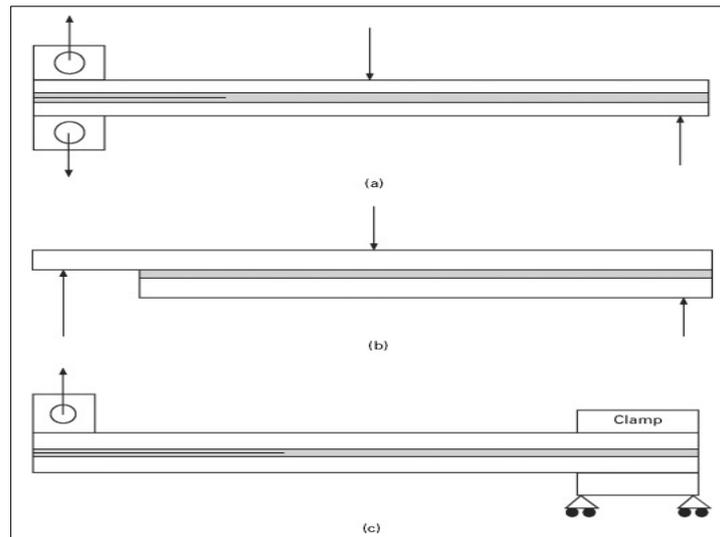
**Fig 10:** Mixed-mode (I/II) adhesive joint test specimens: a) the mixedmode bend (MMB) specimen, b) the mixed-mode flexure specimen and c) the asymmetric double cantilever beam (ADCB), also know as the fixed-ratio mixed-mode (FRMM) specimen
