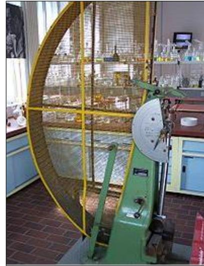
Fig 3: A vintage impact test machine. Yellow cage on the left is meant to prevent accidents during pendulum swing, pendulum is seen at rest at the bottom<sup>[1]</sup>
