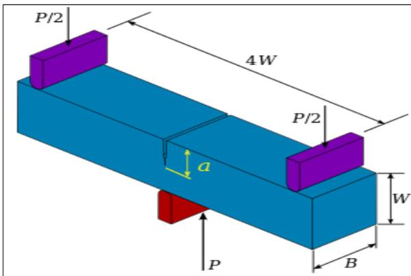
Fig 4: Single-edge notch-bending specimen (also called three-point bending specimen) for fracture toughness testing
