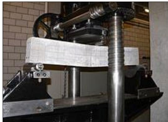
Fig 5: 1940s flexural test machinery working on a simple of concrete
