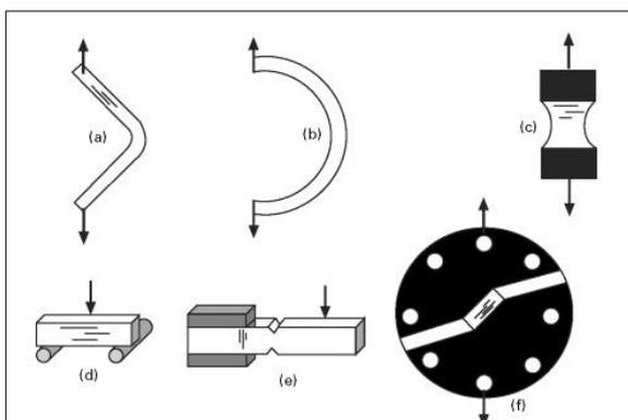
**Fig 9:** Interlaminar strength test specimens. Tension: (a) 90° bend; (b) C- specimen; (c) ILTT. Shear: (d) ILSS; (e) Iosipescu. Tension and shear: (f) Arcan fixture
