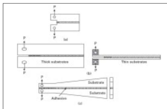
**Fig 1:** Cleavage and fracture tests; (a) compact tension, (b) double cantilevered beam, (c) tapered double cantilevered beam
