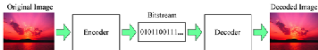
Fig 1: The basic flow of image compression coding
