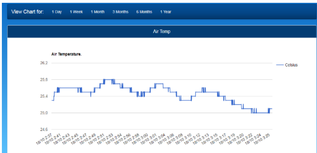
Fig 4: Screenshot of the proposed WiFi monitoring system with plotted measurement results of air–temperature by using AM2315 sensor.
