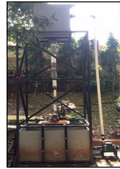
Fig 6: Pump testing device as a turbine
