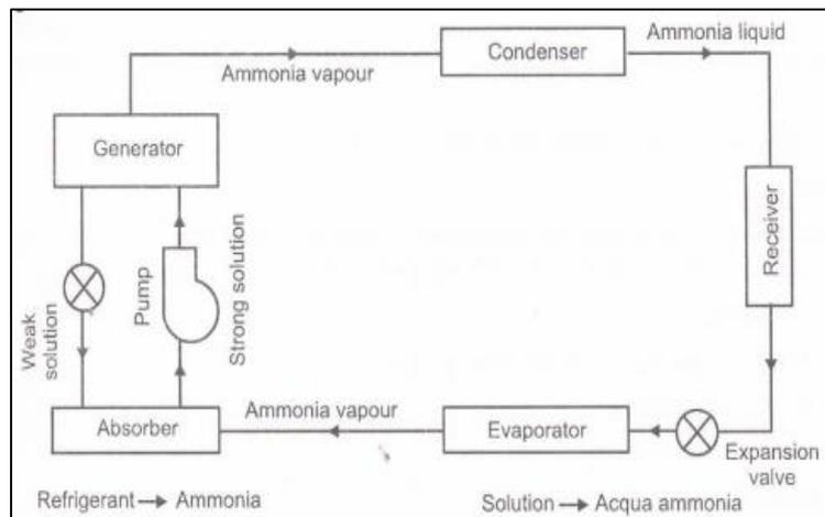
Fig 4: Vapour Absorption System Diagram
